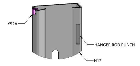
2. MOVE THE H12 INTO POSITION. USE THE SPACER AS A GUIDE BETWEEN THE HEAD STOP OF THE FRAME AND THE H12. USING THE THICKNESS OF THE INSTALLATION KEY, POSITION THE HINGE HOUSING TO THE HEAD OF THE FRAME. INSTALL THE H12 HINGE HOUSING AS INSTRUCTED.
